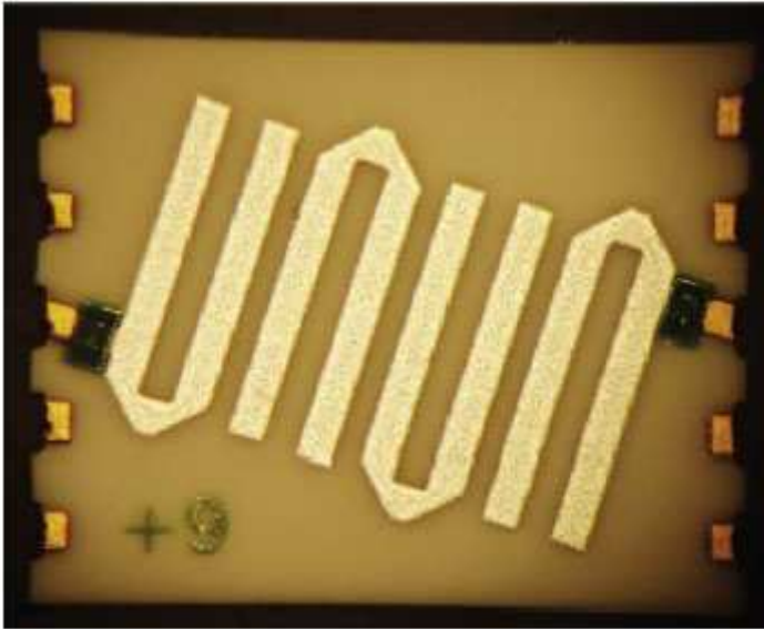
4. This bandpass filter requires low insertion loss across its 400-MHz passband. The 6-GHz filter was fabricated with PCTF technology to reduce size while meeting electrical performance goals. (Photo courtesy of Multispectral Solutions, Inc., Germantown, MD.)
