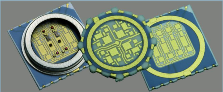
\* **25-125  $\mu\text{m}$  Cu on  $\text{Al}_2\text{O}_3$ , AlN, BeO**
