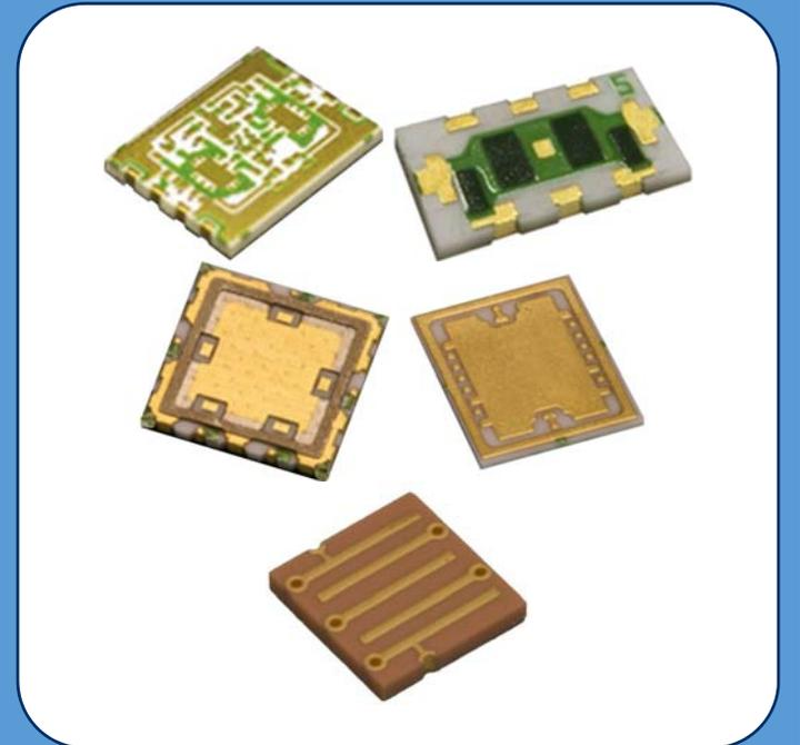
Leadless SMT Substrates / Packages on alumina, AlN, BeO and Barium Titanate with PCTF metallization (25-50  $\mu\text{m}$  thick copper), solid metal plugged vias and castellations, printed thick film resistors, Ni-Au finish and selective gold tin plating for RF Power Amplifiers, LNAs, attenuators and filters.
