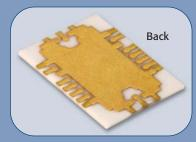
**A .4x.5" hermetic SMT substrate** for direct PCB mount for **5 W HPA**. PCTF metallization with .002" copper and thermal vias under the GaAs die enabled a compact power package with a thermal resistance below 1°C/W. Low inductance interconnects allow operating at 6 GHz with insertion losses below .3dB. (Courtesy of IAI Elta Systems)
