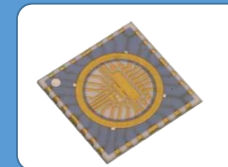
LED sensor: Leadless SMT package for direct PCB mount with 25µm Cu on BeO, metal plugged via holes, castellations and multilayer dielectric.
