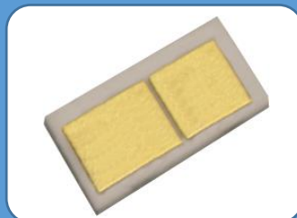
AlN ceramic carrier with copper metallization and Ni-Au finish for an LED with pad down design (50µm gap) for a high volume application.
